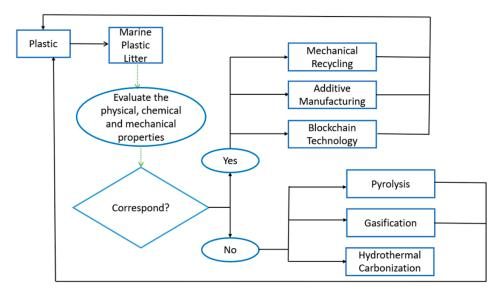
Figure 1. Scheme for recycling of marine plastic litter.
