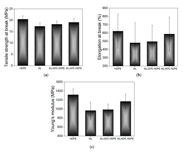
**Figure 2.** Mechanical properties of marine plastic litter containing varying percentage of HDPE (0–40 wt%) compared with those of virgin HDPE. (**a**) Tensile strength at break; (**b**) elongation at break; (**c**) Young's modulus. Adapted from [71].
